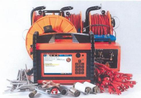
Automatic System for Resistivity and IP Imaging
